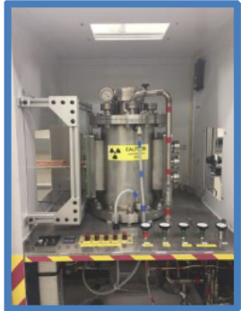
Compact Fuel Element Environmental Test (CFEET)
