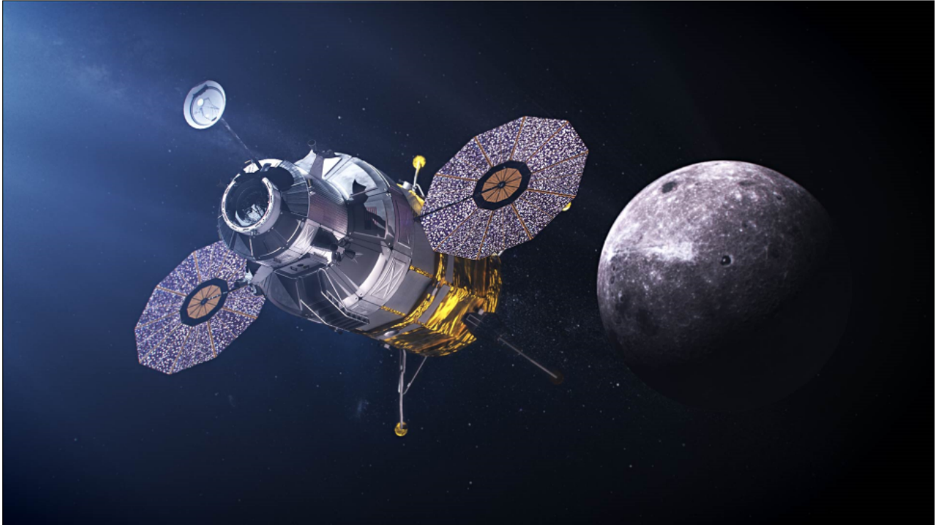
Figure 1: NASA's government concept for a Human Landing System includes an ascent, descent, and transfer module.
