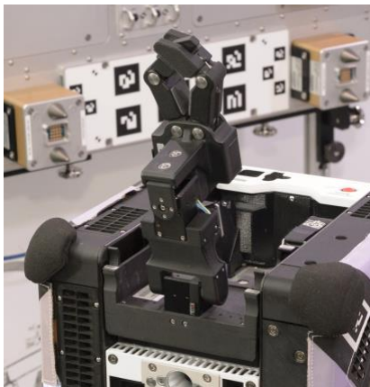
Fig. 4: Astrobees's Perching Arm in phase of deployment, mounted in the top payload bay.
