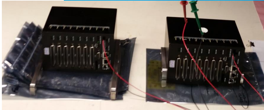
UEI Data Cubes [Thermocouple Signal Conditioning]
