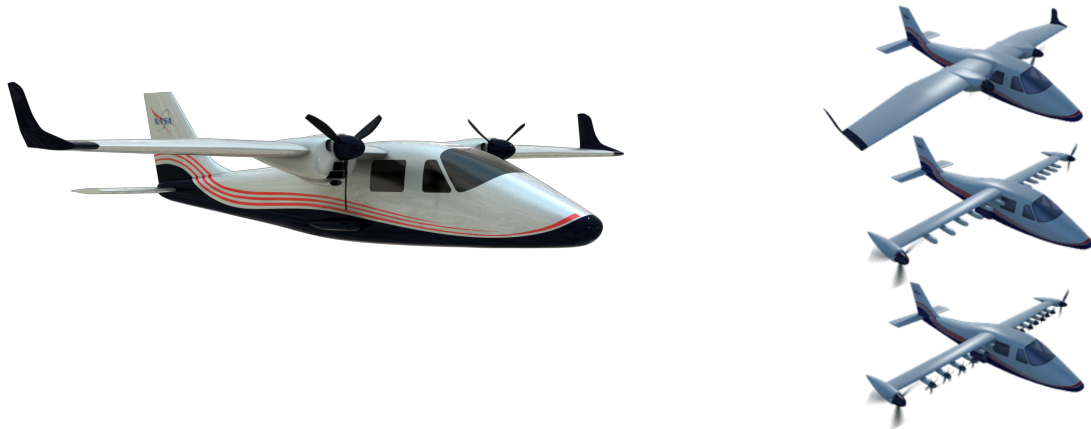
Figure 1. NASA’s X-57 “Maxwell” Aircraft, (Left) Mod #2 Variant, (Right) Evolution of Mod #2, 3, & 4 Variants
