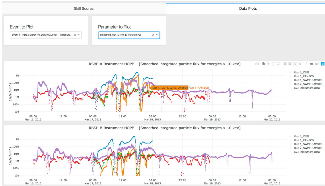
Figure 4. Comprehensive Assessment of Models and Events Using Library Tools plots of fluxes observed and modeled at the RBS-P-A and RBS-P-B locations. Point picking is showing a value along one of the model tracks. RBS-P = Radiation Belt Storm Probes; HOPE = Helium Oxygen Proton Electron.
