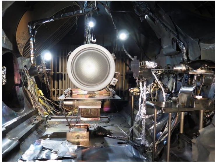
Figure 1: NEXT engine mounted in EP2 for steady-state characterizations.
