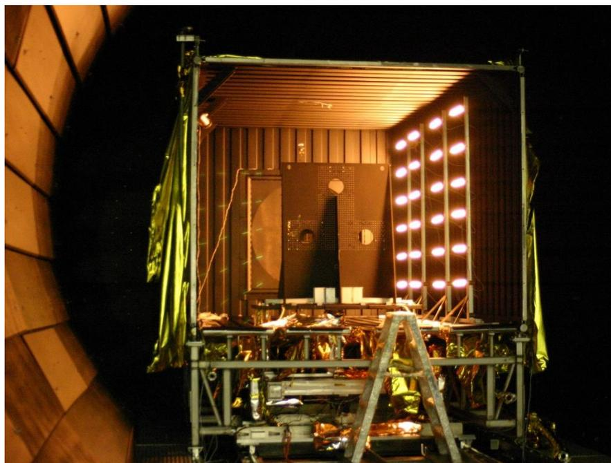
Solar lamp array consists of 24 lamps connected in a 3-phase delta configuration (8 per phase).
