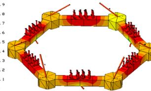
Reaction structure with insulation radiates to cold enclosure  $e=0.05$
