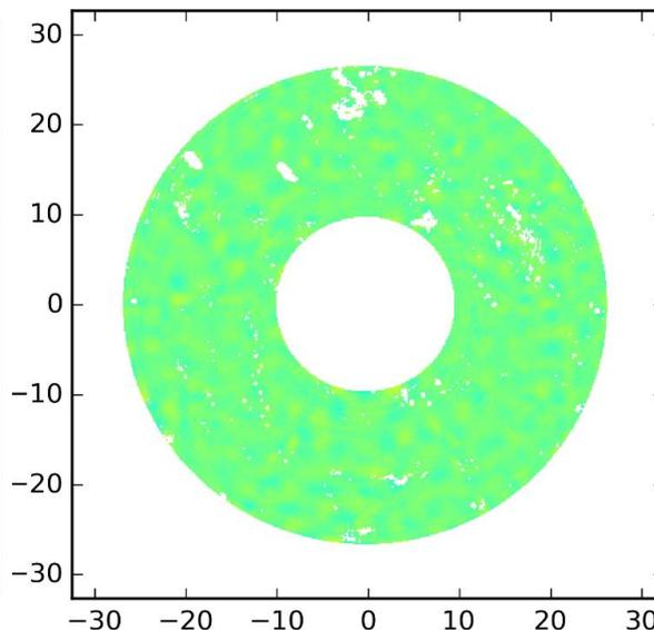
Correlated Map was produced by introducing lateral strain difference between front/back sheets.
