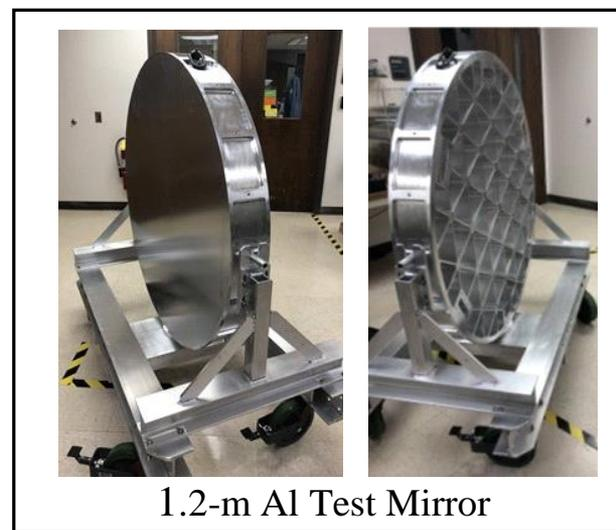
Thus, PTC procured a 1.2-m aluminum mirror to serve as a pathfinder test article. Since aluminum has a larger CTE than ULE<sup>®</sup>, it is expected to provide a 2X larger signature – which can be used to practice the PTC control algorithm.
