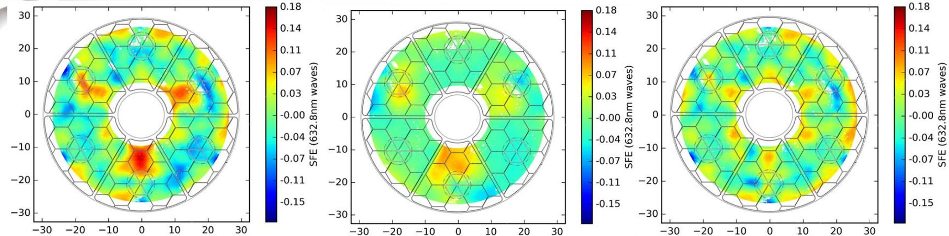
Measured = 28.8nm rms    −    Model = 17.7nm rms    =    Residual error = 22.8nm rms
