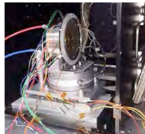
Ultra-Stable pm-scale mirror assembly functional testing with surrogate fused-Si substrate
