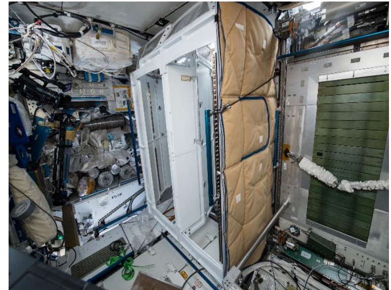
Toilet Stall deployed on ISS Node 3 – modular panels allow partial removal for maintenance in adjacent racks
