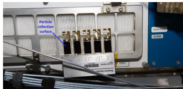
Fig. 1. Passive Sampler J is mounted on the edge of the HEPA filter in the US Lab in ISS during the Aerosol Sampling Experiment in Increment 50/51
