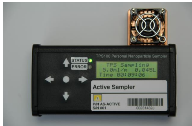
Fig. 2. The Active Aerosol Sampler is the modified COTS TPS100™ Personal Nanoparticle Sampler
