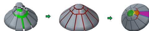
Figure 1. HEEET integration with the carrier structure. Molded and resin infused tile panels are bonded and routed precisely for integration of seam between the acreage tiles.
