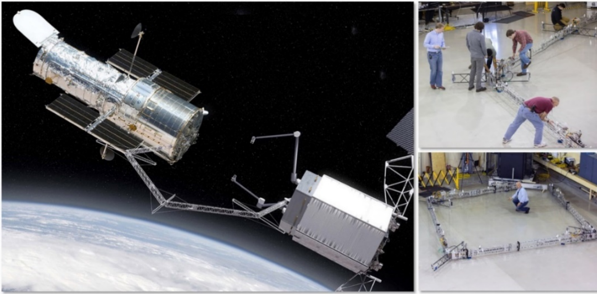
Figure 14. An artist's rendition of TAIMAN servicing the Hubble Space Telescope (left). The first test series of the CIRAS TALISMAN 20 meter (four link arm) demonstrations in the flat floor facility of the LaRC Structures and Materials Lab (right). 65
