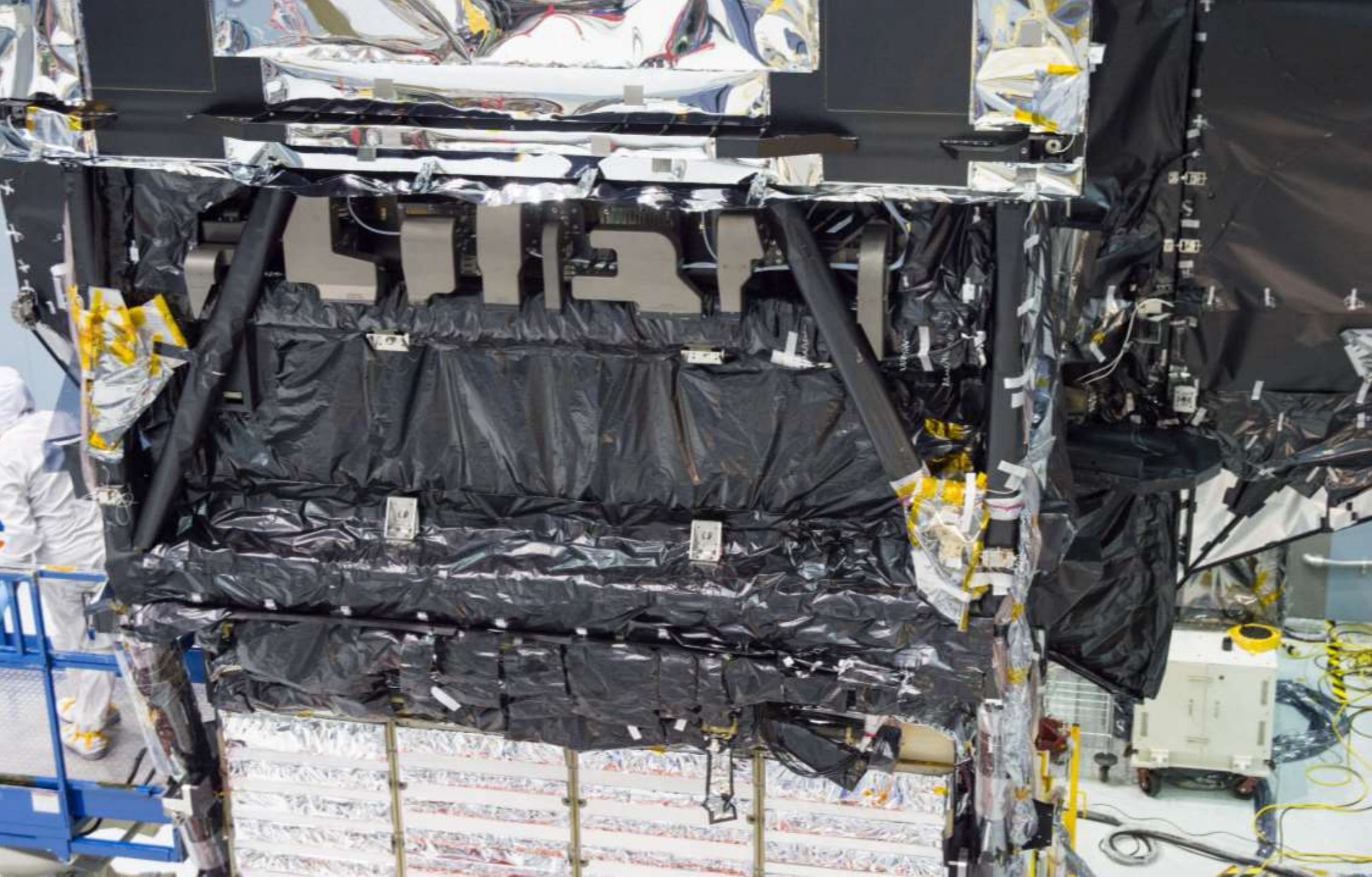
Harness Radiator (HR) Integration
