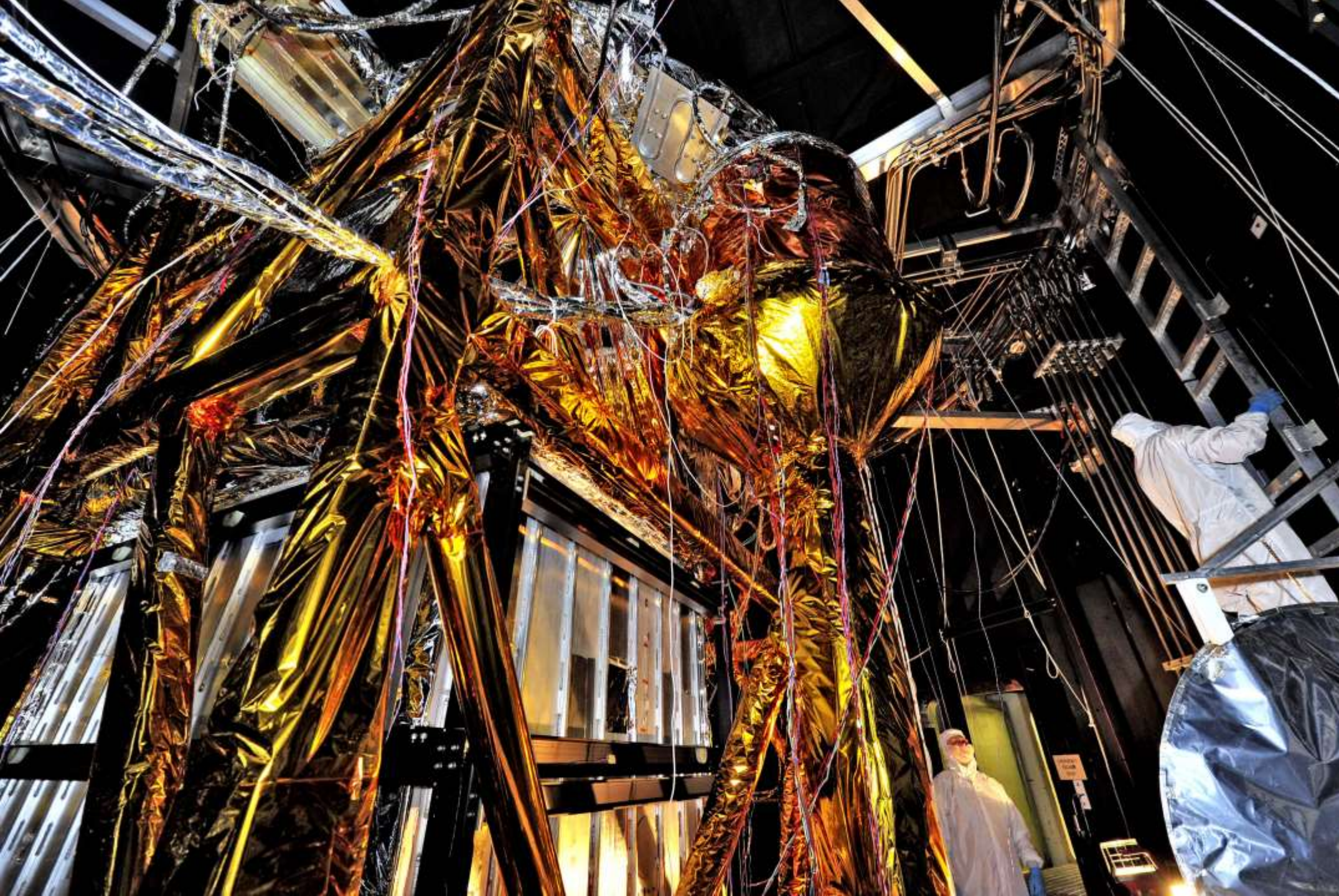
ISIM in the thermal vacuum chamber
