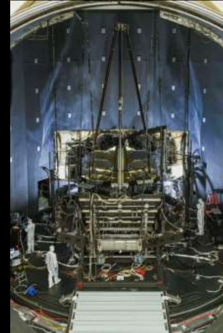
Thermal Pathfinder: Verified all thermal environment/boundary conditions (e.g., sunshield layer 5 thermal simulator, ISIM radiator sinks)
