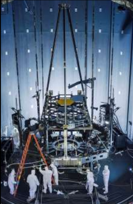
Optical Ground Support Equipment (OGSE) #1: Prove-out optical GSE. Featured Cryo Optical Test on Pathfinder OTE w/ 2 Spare PMSA's and Spare Secondary
