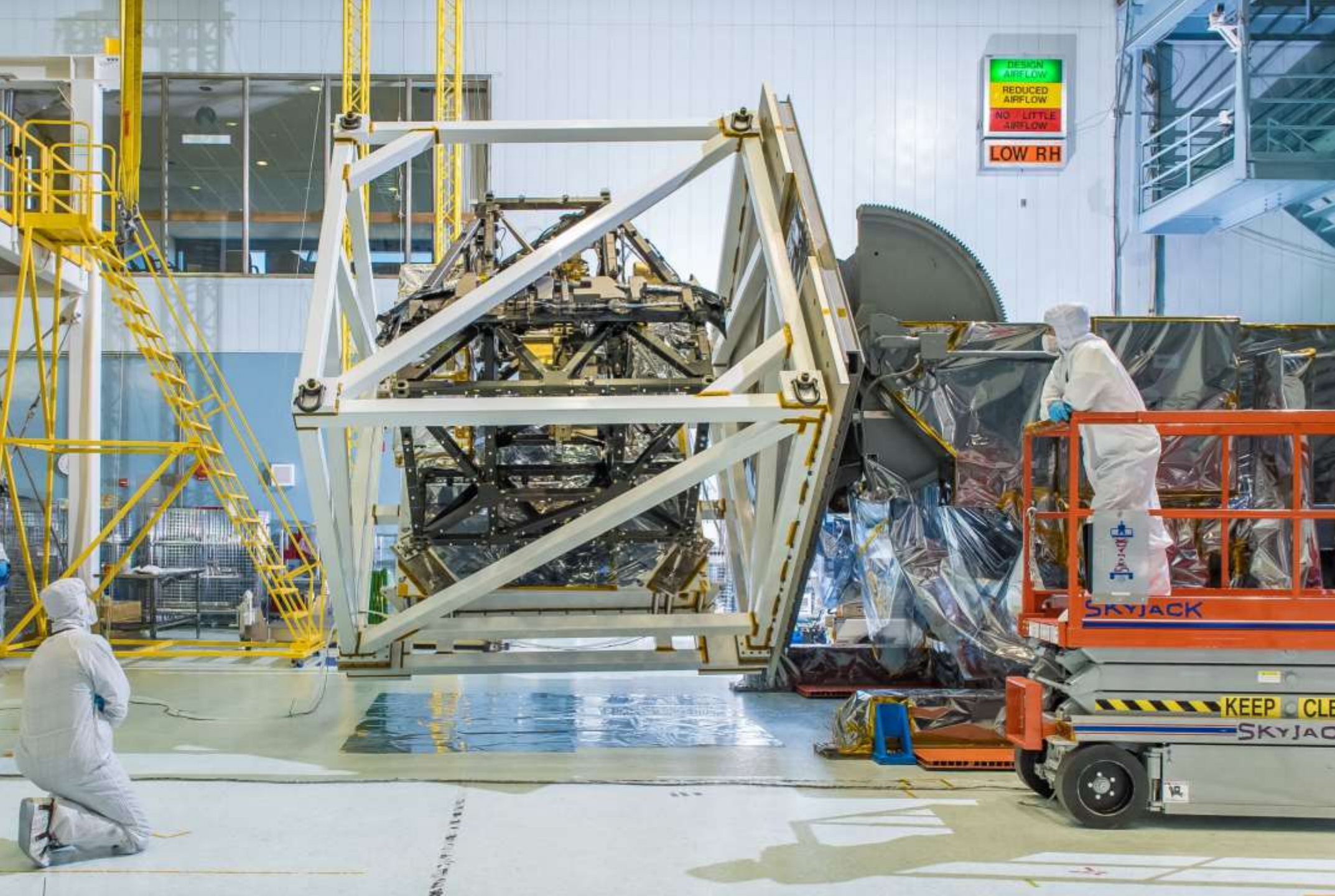
ISIM Gravity Release Test
