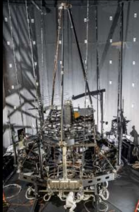
OGSE #2: 2 nd Cryo Optical Test but w/ Flight Aft Optics System and AOS Source Plate Assembly. Full check-out of optical GSE and measurement schemes
