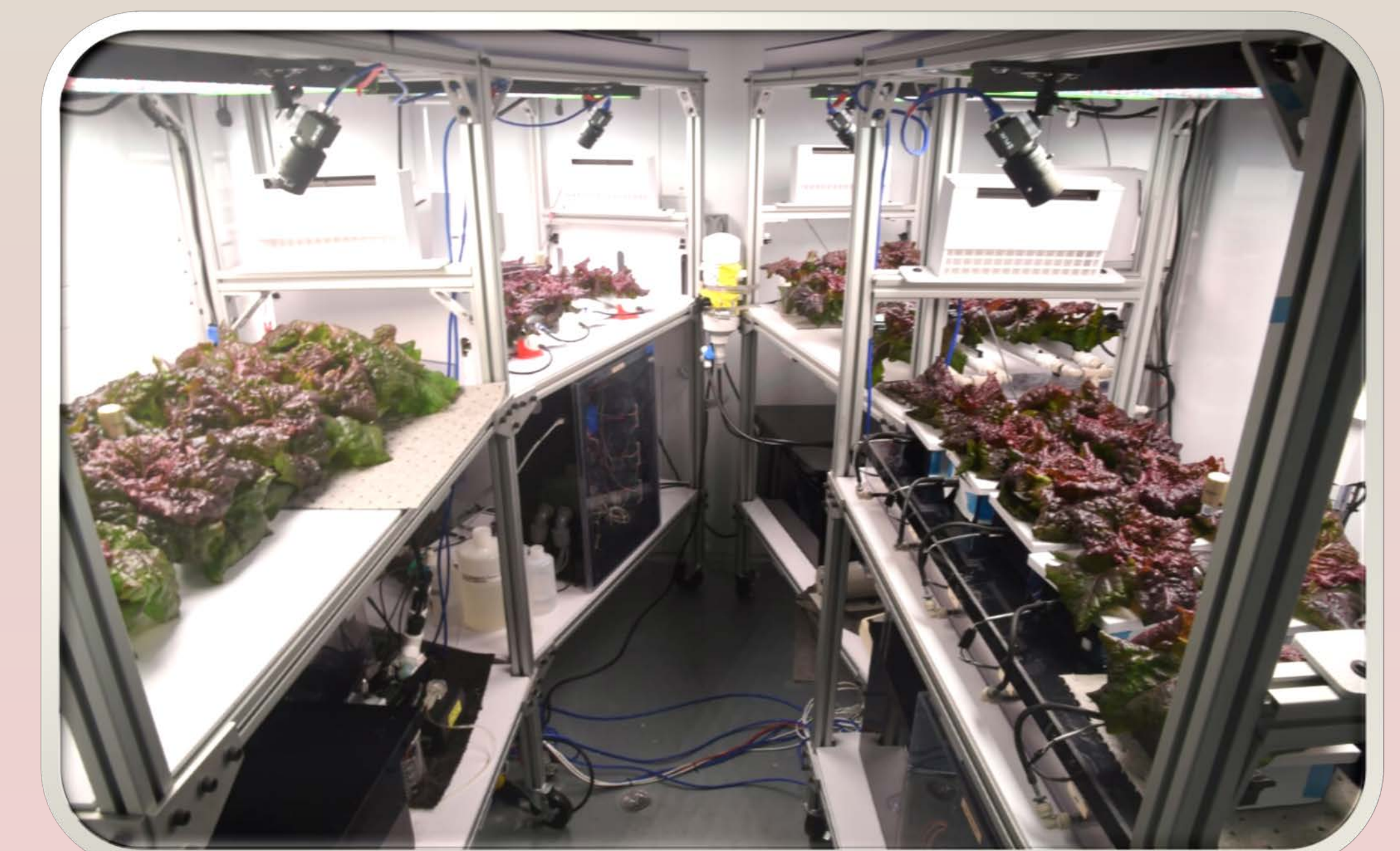
Figure 4. NFT (bottom left), Passive PTNDS (Top left), Active PTNDS (Top right), and On-Demand (bottom right)
