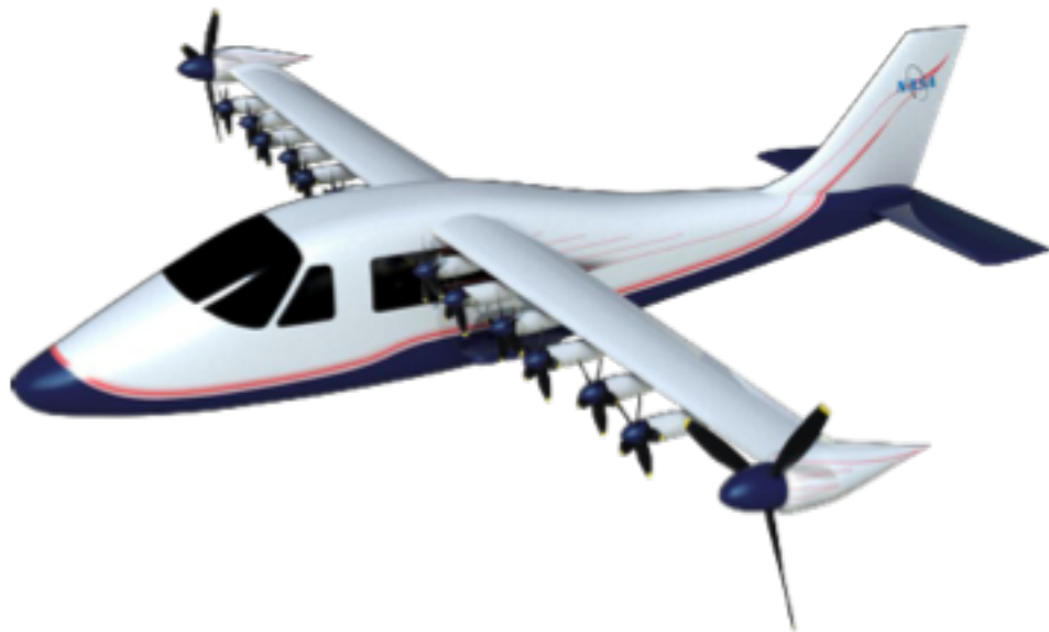
Figure 7, A Representation of the X-57 SCEPTOR as a Re-Winged Tecnam P2006T
