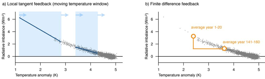
SM Fig. 2: Schematic of feedback definitions
