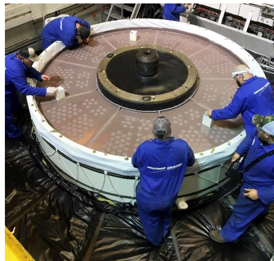
Fig. 12. Artemis II solid rocket motor segment casting
