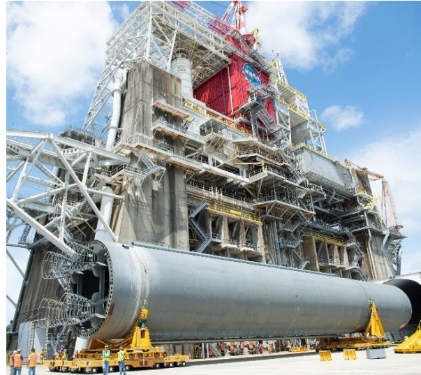
Fig. 9. Core stage pathfinder at Stennis B2 stand
