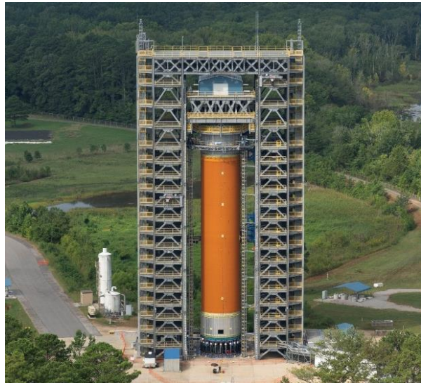
Fig. 7. LH 2 structural test article in test stand
