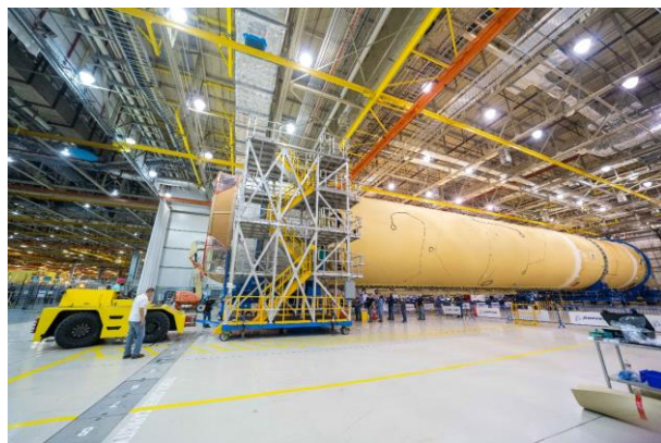
Fig. 6. Artemis I engine section and core stage mate
