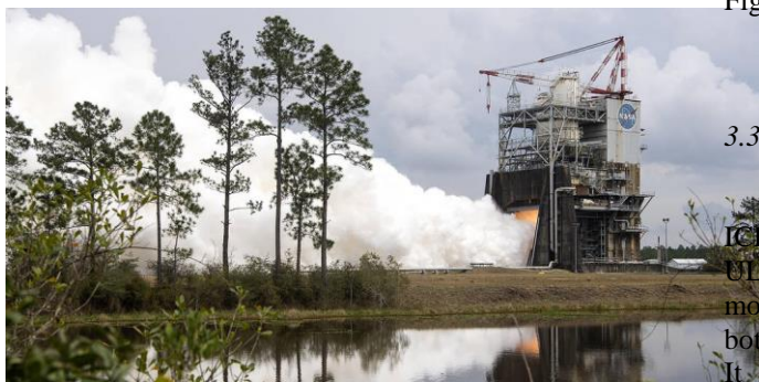
Fig. 11. RS-25 hot-fire test at SSC
