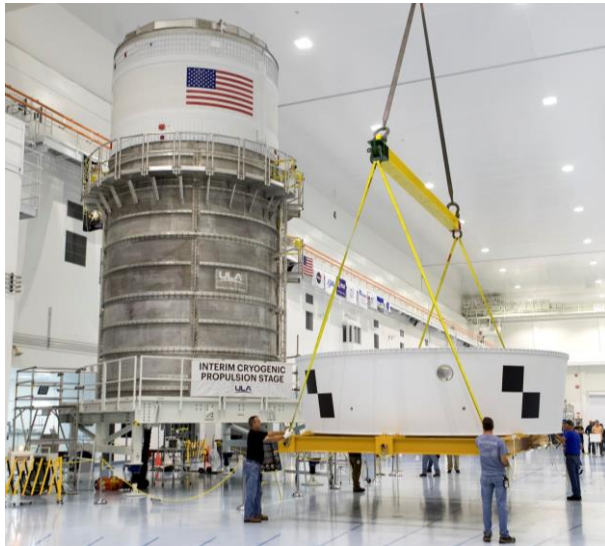
Fig. 13. Artemis I ICPS and OSA ready for integration at KSC
