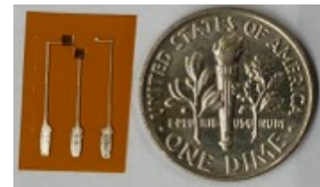
Printed cortisol sensor
