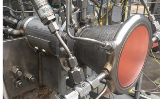
Fig 13. Bimetallic LWDC nozzle at MSFC TS115.
