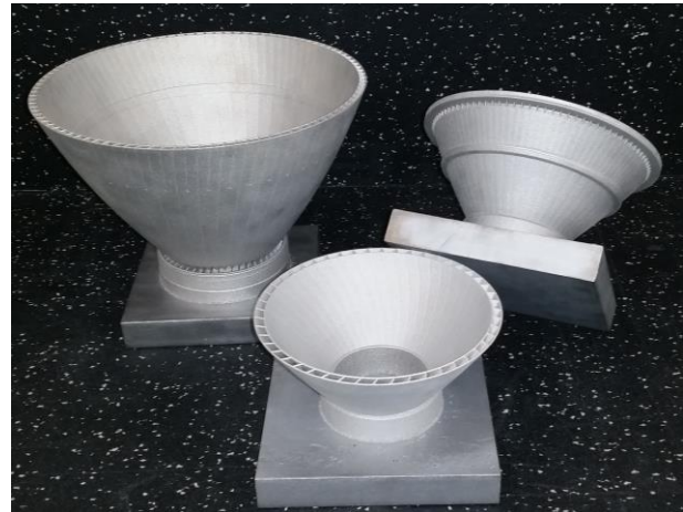
Fig. 9. Examples of Blown Powder DED integral channel nozzles (RPMI).
