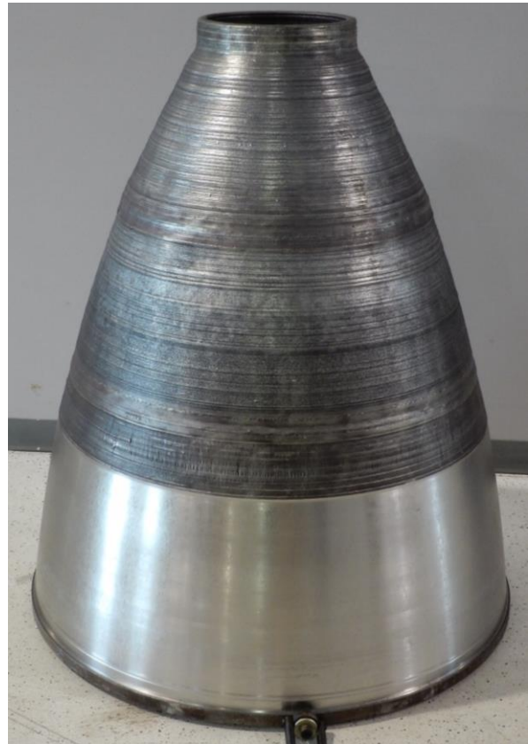
Fig 18. 1/2-Scale RS25 Nozzle Liner fabrication with Blown Powder DED, No channels. (approx. ~44” dia and ~48” tall)
