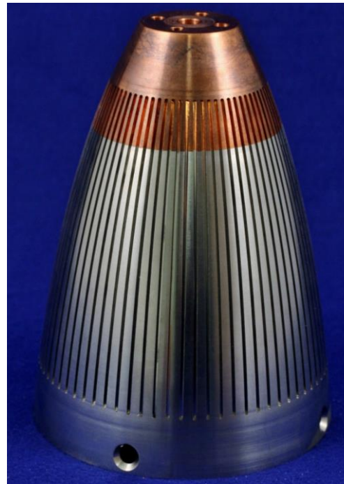
Fig. 11. Explosive bonded axial bimetallic liner.
