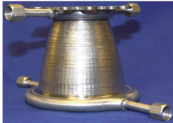
Figure 4. LWDC Closeout of Monolithic, Inco 625.
