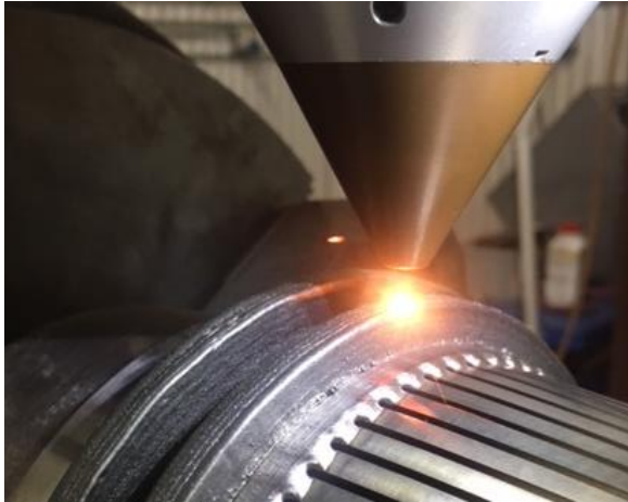
Fig. 7. Blown Powder DED process applying nozzle manifold preparations.
