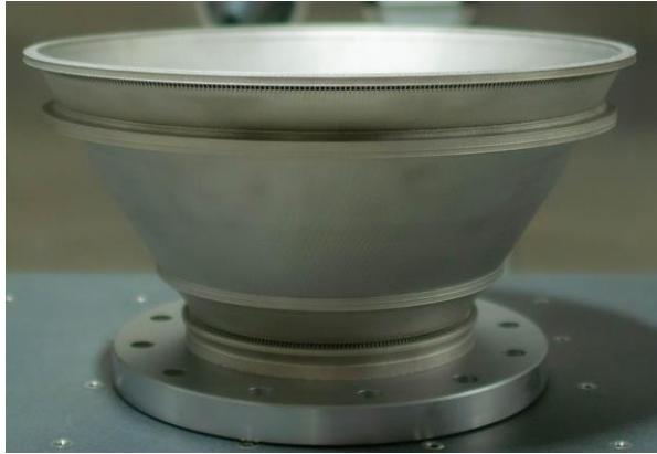
Fig 19. JBK-75 Integral-channel DED 35K-lbf nozzle fabricated at RPMI.
