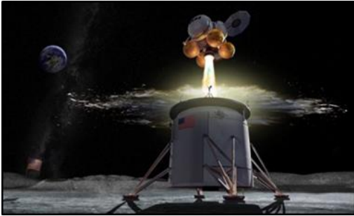
Fig. 2. One concept for a 2024 human lunar lander. Both descent and ascent stages are shown.
