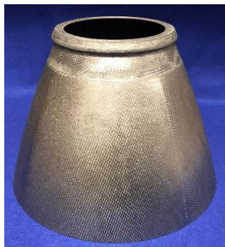
Fig. 16. Carbon-Carbon Advanced Technologies (C-CAT) SiC-enhanced C-C.
