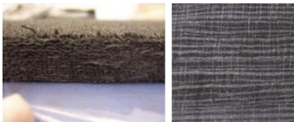
Fig. 7. Left: Example of a needled, carbonized, lyocell plate preform. Right: Through-the-thickness view of a needled lyocell-based composite plate.
