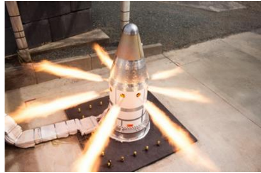
Fig. 5. Orion LAS ACM Qualification Motor-1 (QM-1) test on 20 March 2019 at Northrop Grumman Innovation Systems (NGIS) facility in Elkton, Maryland. The system was also more recently successfully demonstrated with the Orion LAS Ascent Abort-2 (AA-2) flight test on 2 July 2019.
