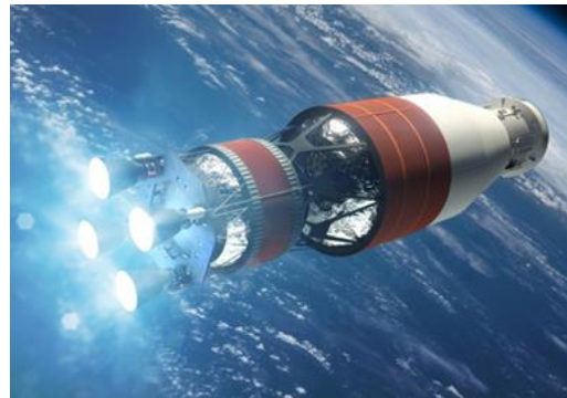
Fig. 1. Space Launch System (SLS) Exploration Upper Stage (EUS) with RL10C-3 engines.
