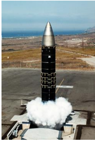
Fig. 4. US Air Force Peacekeeper ICBM test flight. The Boeing led program included 50 test flights. Stage III of the missile had a C-C extendible exit cone.
