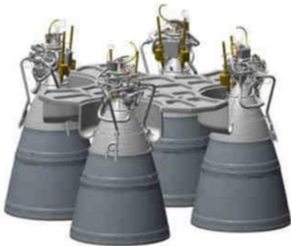
Fig. 3. Four RL10C-3 engines in SLS EUS configuration. Each nozzle extensions consists of a fixed (non-translating) carbon-carbon “A” plus “B” cone set.
