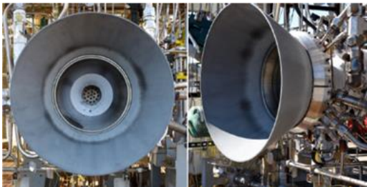
Fig. 19. Two post-firing views of the C-CAT SiC-coated PAN-based C-C.
