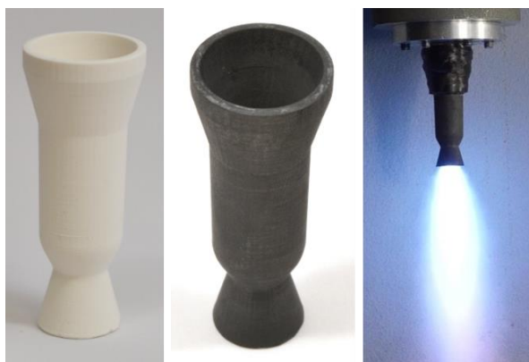
Fig. 11. Left: Subscale 3D printed reinforced pre-ceramic polymer combustion chamber / nozzle component. Center: Same component after matrix pyrolysis. Right: Hot-fire test at Vector Launch.
