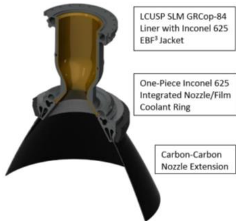
Fig. 17. LCUSP thrust chamber assembly with C-C composite nozzle extension attached.
