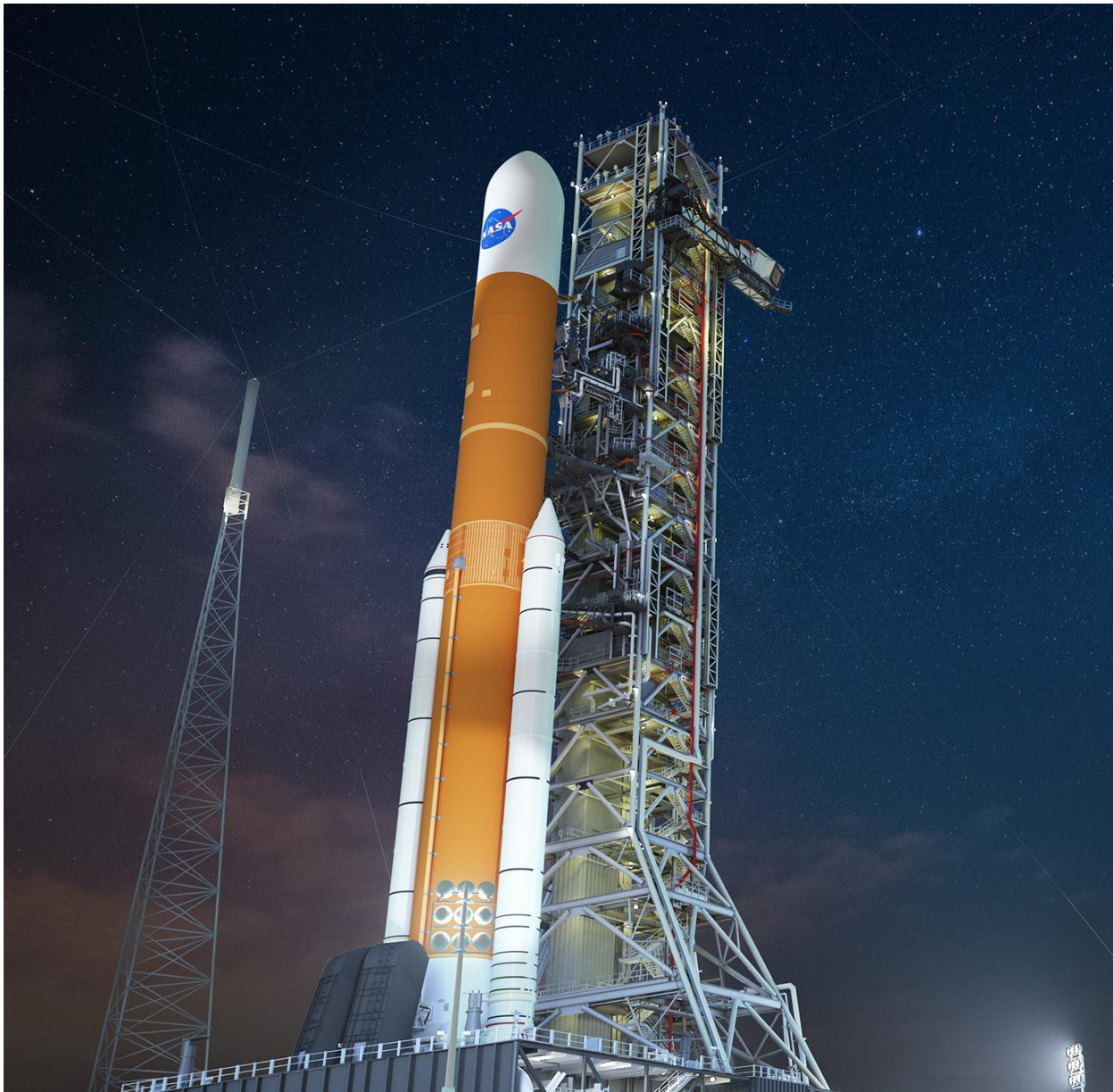
Figure 1. Artist's rendering of SLS Block 1B with an 8.4 m-diameter fairing on the launchpad
