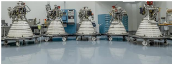
Figure 7. Five RL-10 upper stage engines are complete for future SLS missions
