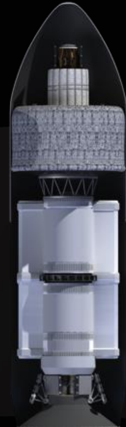
10m fairing w/notional Mars payload
