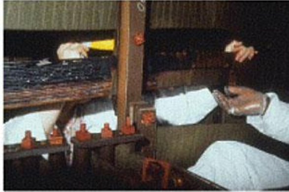
Permanent damage to the Salem New Jersey Nuclear Plant GSU Transformer caused by the March 13, 1989 geomagnetic storm. Photos: PSE&G
