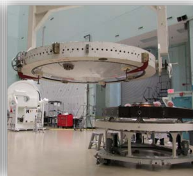
Removal of Spare PM from Aft Metering Structure May 2019
