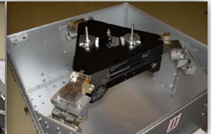
Secondary Mirror Support Structure (SMSS) ready for re-use
