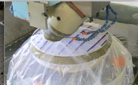
In process shaping of SM to WFIRST prescription
