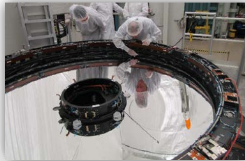
Removal of PM Scraper 7/2018
