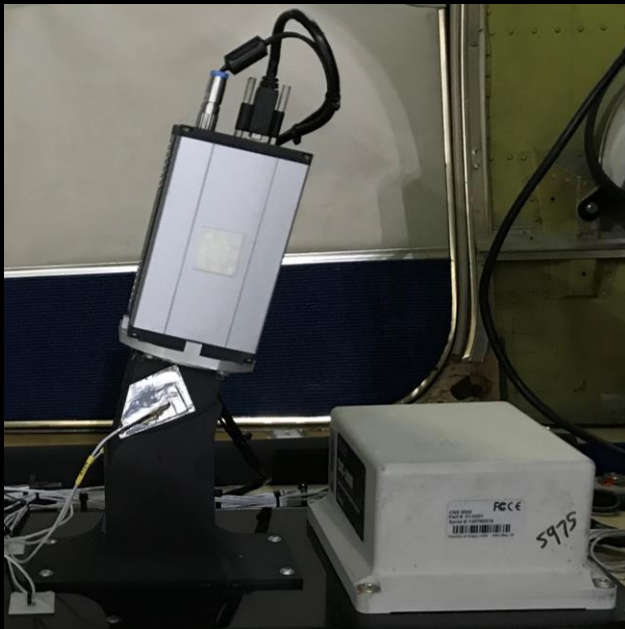
Installation on Twin Otter with INS and temp sensors
