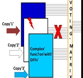
Block diagram of block TMR (BTMR): a complex function containing combinatorial logic (CL) and flip-flops (DFFs) is triplicated as three black boxes; majority voters are placed at the outputs of the triplet.
