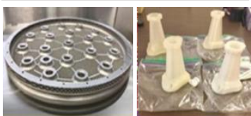
ISM Design Database Development Life Support Systems Retaining Plate (Left); Logistics Reduction Urine Funnels (Right)
