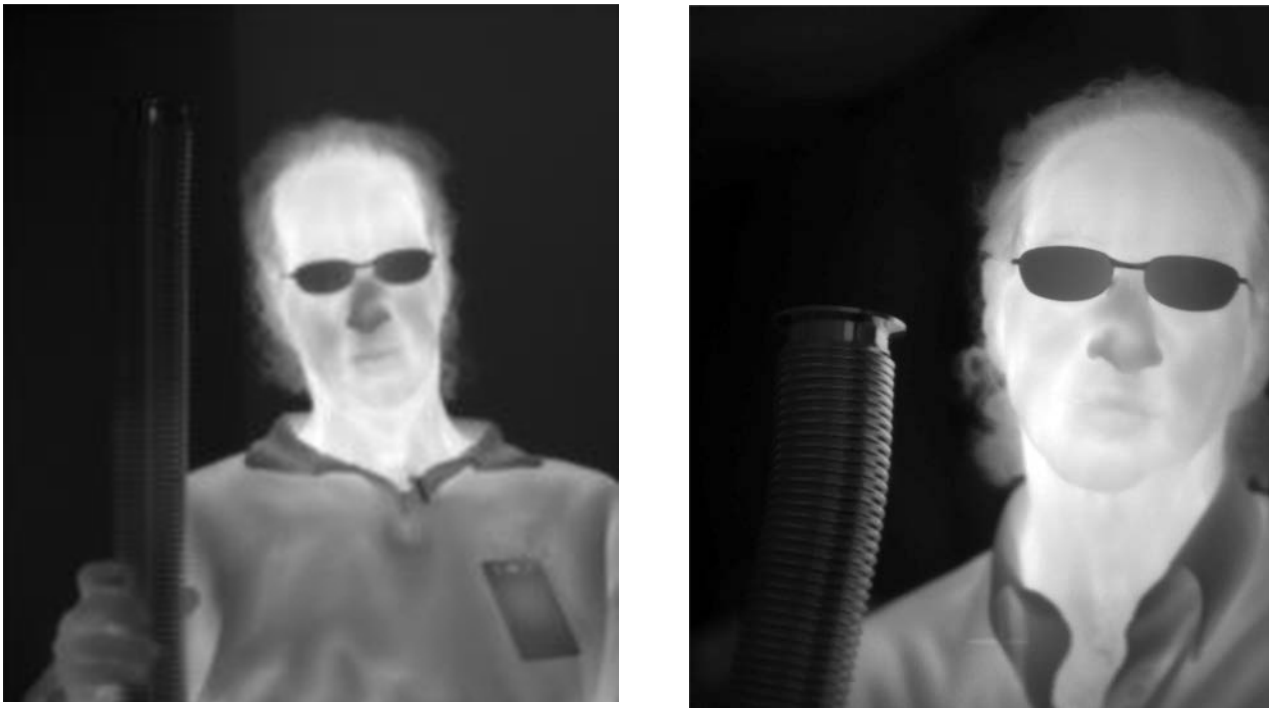
Figure 5. Left; QWIP narrow band image. Right; First SLS broadband IR image taken in the Goddard lab. Subjectively, the images looked comparable but the integration time for the SLS image was almost 90 times shorter than for the QWIP image due to the increased sensitivity (0.19 ms vs 16.65 ms).
