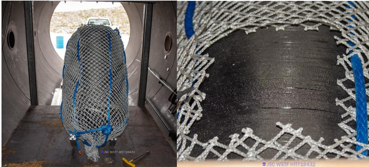
Figure 5 Overall front view of sample secured within the target tank (left) and close-up view of desired impact location with Dyneema mesh window cut (right). Both images taken prior to wood blast mitigation installation.
