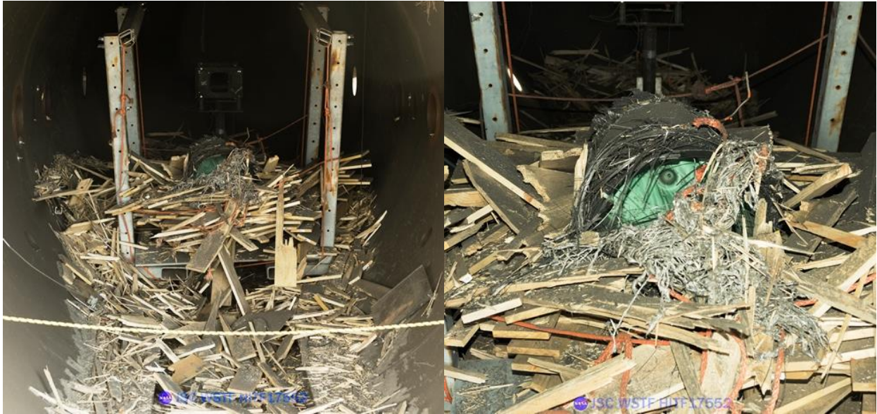
Figure 13 Overall rear view of damage adjacent to test fixture within target tank (left) and close-up view of damage present within the test fixture as a result of HITF17552 (right).
