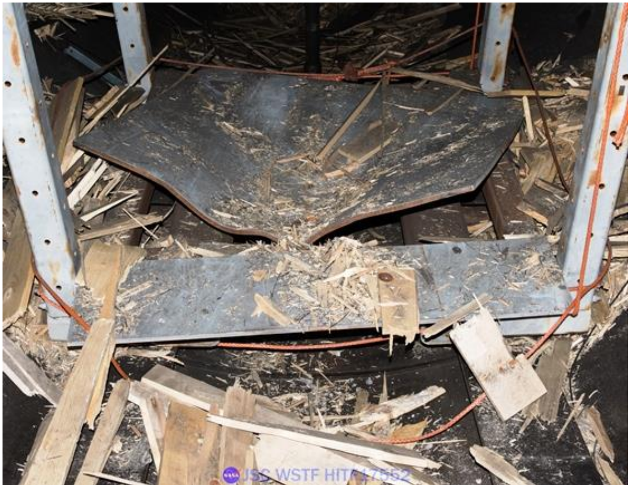
Figure 14 Close-up rear view of damage to test fixture with 16mm thick steel base plate visible HITF17552.
