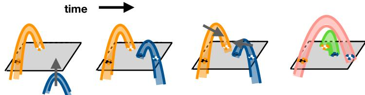
Using active region pairs as a laboratory for measuring reconnection: If each active region is a distinct magnetic system, any new flux linkage between two must be a result of coronal reconnection.
