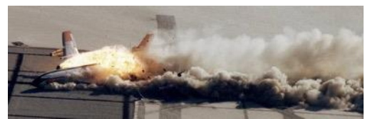
Federal Aviation Administration (FAA) teamed with NASA on Controlled Impact Demonstration (CID) employing a remotely piloted Boeing 720
