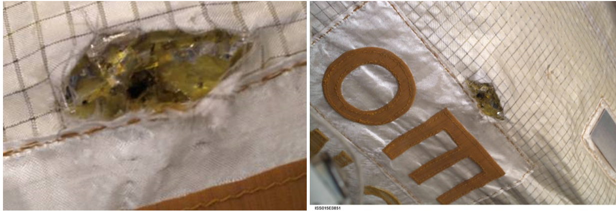
Fig. 16. FGB compressor thermal blanket MMOD damage.
