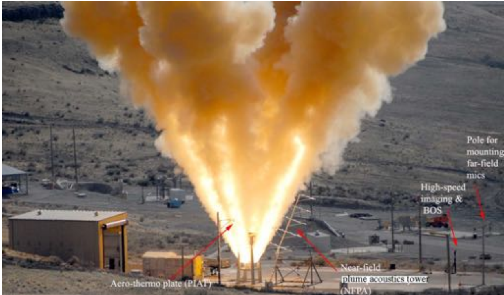
Picture from ST1 abort motor ground test
