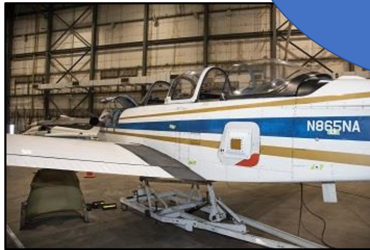
Array Mounted to T34-C in Hanger at Armstrong Flight Research Center
