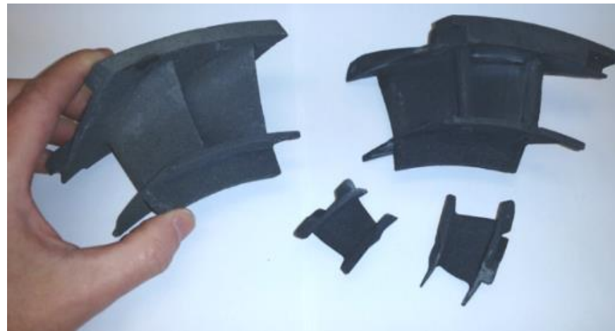
High pressure turbine cooled doublet vane sections.
