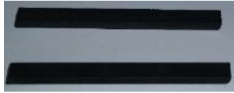
Bend bars for strength testing
