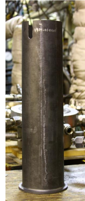
SiC/SiC Combustion Liners: Outer Liner and EBC Coated Inner Liner
