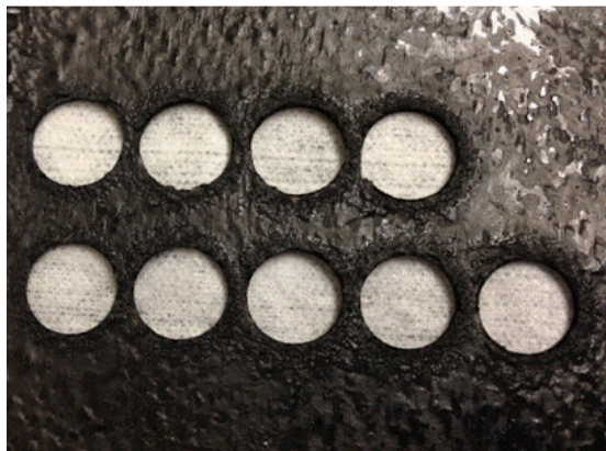
SEM specimens cut with different laser power/speeds
