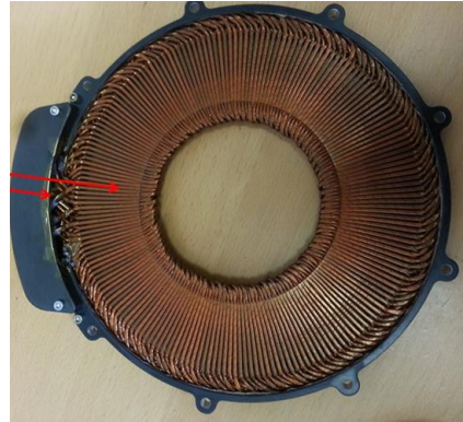
Litz Wire Coreless Stator
