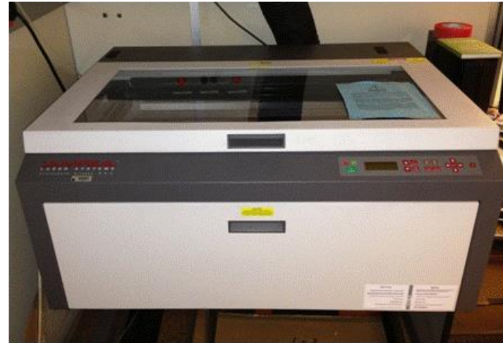
Universal Laser System (Two 60 watt laser heads and a work area of 32"x18")
