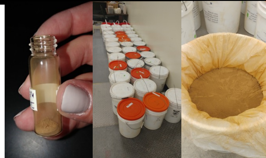
JSC Rocknest (left to right): prototype simulant, 5-gallon buckets of USGS-produced simulant, JSC Rocknest
