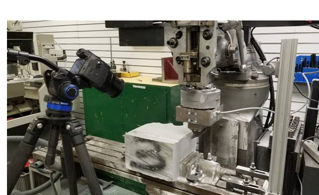
Left to Right: Single-pick test stand with gypsum block; single-pick test; two excavated lines; 3D scan of excavated lines to measure excavated volume
