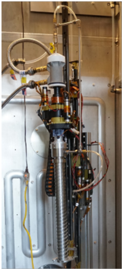
Honeybee Robotics Planetary Volatile Extractor (PVEx) Drill (left) and concept for Extraction of Water from Mars' Ice Deposits (right)
