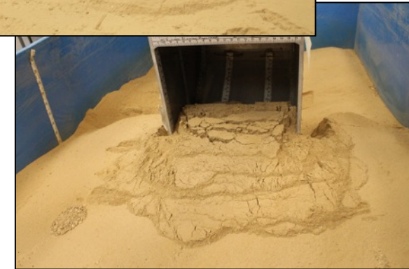
Top Left: Excavation lab at NASA GRC; Top Right: Bow wake in lightly compacted-simulant; Right: Bow wake in highly-compacted simulant
