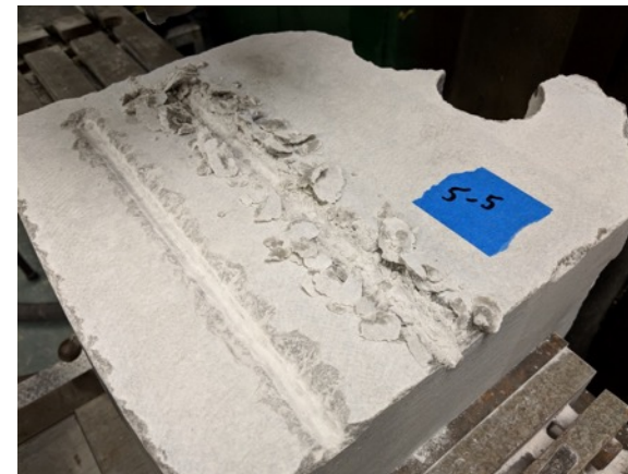
Left to Right: Single-pick test stand with gypsum block; single-pick test; two excavated lines; 3D scan of excavated lines to measure excavated volume
