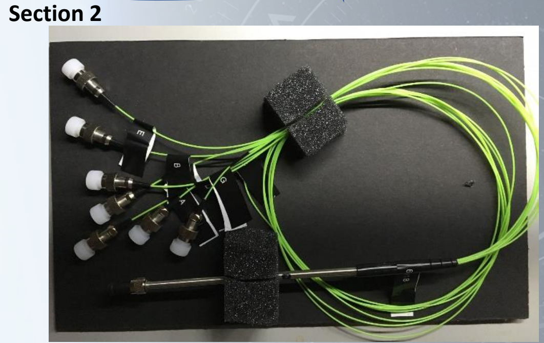
A packaged 7:1 FMF photonic lantern.
