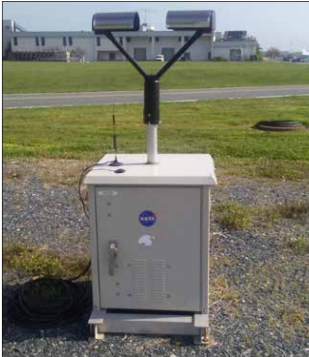
Automated Parsivel Unit (APU) deployed at NASA's Wallops Flight Facility. The Parsivel disdrometer itself is shown atop the computer and electronics container. The small antenna is a GPS. The APUs were designed at NASA's Marshall Flight Facility for remote operations of the Parsivel instruments.
