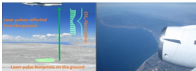
MELI principle of operation (left). DC-8 over the Pacific Ocean during a MELI flight in October 2015 (right).
