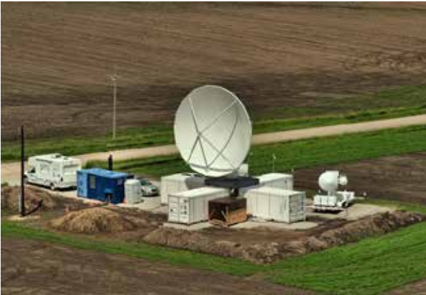
NASA's NPOL radar deployed during the Iowa FLOODs Study (IFLOODS) in central Iowa (May–June 2013). The antenna's diameter is 8.5 m (28 feet) and operates at S-band (10 cm) with an output power in excess of 800 kW
