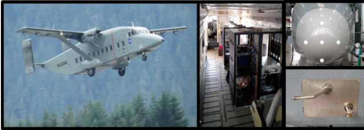
The CARAFE is installed on the Sherpa aircraft (left). Payload includes gas analyzers (center), nose radome modified for the 3-D wind system; pressure ports highlighted for clarity (upper right), and fuselage plate holding angle-of-attack and true air temperature probes (lower right).
