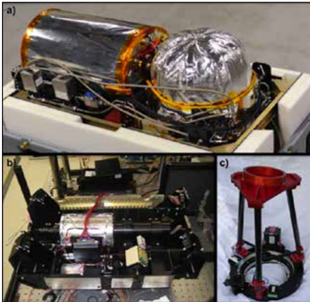
A picture of (a) the current ACATS instrument includes (b) the receiver subsystem and (c) the telescope subsystem.
