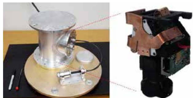
Photograph of the AirHARP structure and doghouse. Everything is contained within the doghouse, including the data system. The pen on the left hand side shows the scale of the system
