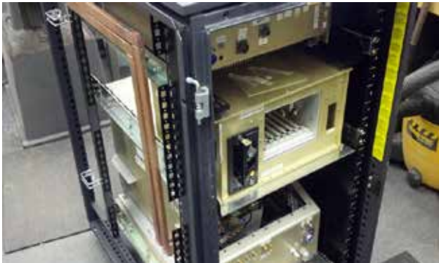
The X-BADGER radar system with digital receiver on top, data system on the middle rack, and transmitter on the bottom with copper waveguide for the two beams on the left.
