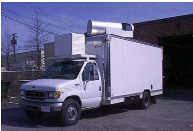
The GLOW mobile Doppler lidar measures wind profiles from the surface into the stratosphere. The two-axis scanner (on the roof) allows full-sky scanning of the lidar
