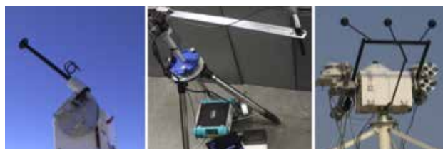
Complementary setup: an additional spectroradiometer (Fig. a) in sun-tracking mode; or in surface bi-directional reflectance mode (Fig. b); and broadband radiometers on tracking station for diffuse and direct components (Fig. c) at various selected wavelength ranges.
