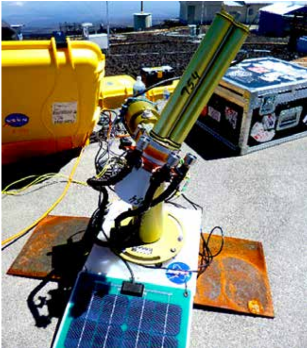
The mini-LHR makes observations of CO 2 and CH 4 at 11,400 feet at Mauna Loa Observatory in Hawaii in tandem with an AERONET sun photometer.
