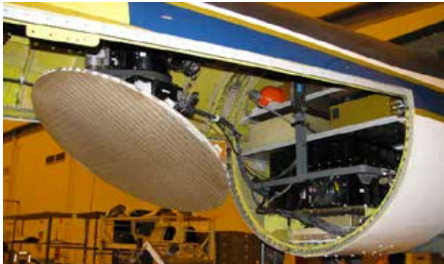
Aft view of EXRAD nose showing transmitter and data system.
