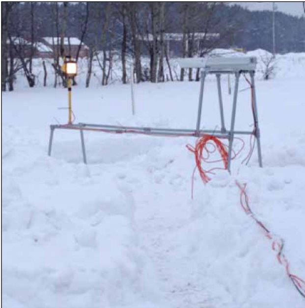
A Precipitation Imaging Package disdrometer shown deployed near Marquette, MI. The PIP was designed by Dr. Larry Bliven at Wallops Flight Facility. It consists of a halogen light and a high-speed camera that are used to image precipitation particles.
