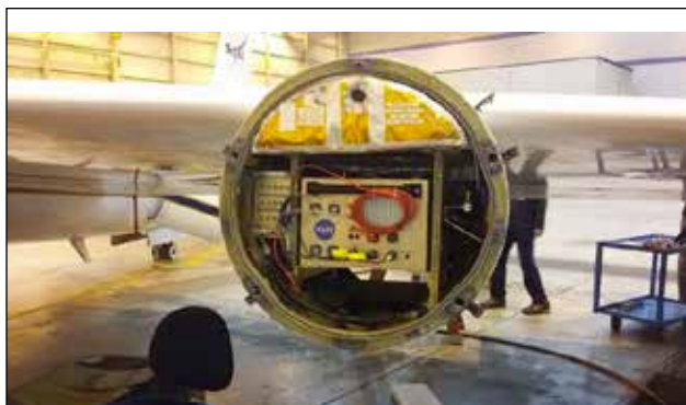
The CAFE instrument installed on the NASA ER-2 at the Armstrong flight research facility in Palmdale, CA. CAFE is easily adapted to fly almost any aircraft.
