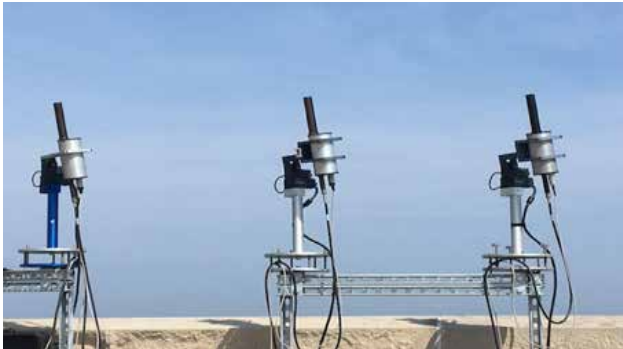
Three Pandora instruments tracking the Sun on the roof of the Chesapeake Bay Bridge Tunnel during the 2017 Ozone Water-Land Environmental Transition Study (OWLETS).
