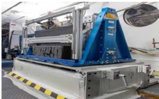
GeoTASO instrument integrated on the NASA LaRC Falcon for the Discover-AQ deployment in Denver (2014).
