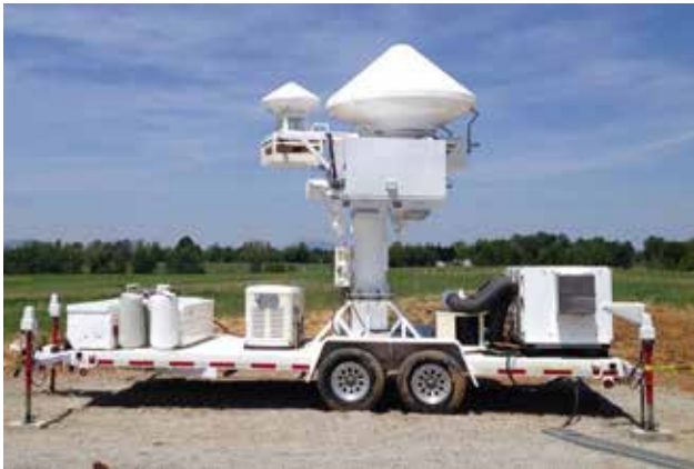
NASA's Dual-polarization, Dual-frequency, Doppler Radar (D3R), currently deployed at NASA's Wallops Flight Facility on Wallops Island, VA.
