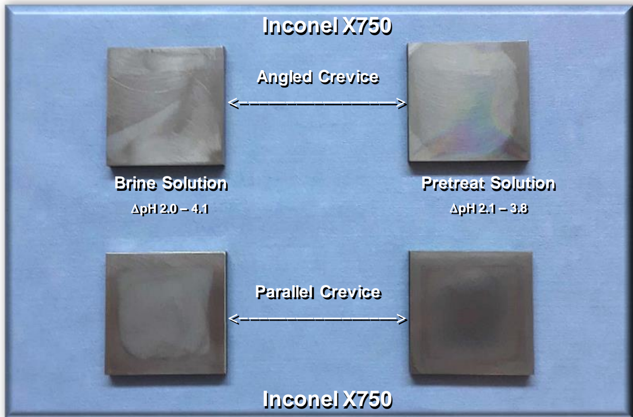
Figure 4: Descriptive images of X750 crevice samples after one year immersion in the subject test solutions revealing clean, undisturbed surfaces corresponding to microscopic analysis.
