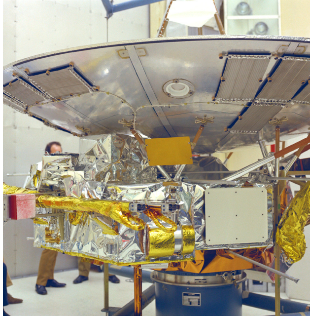
Figure 4. This image shows pressurized gas cells on the back of Pioneer 10's antenna as it's being readied for its mission.
