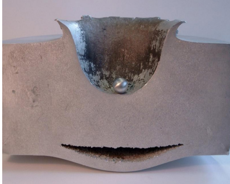
Figure 39. The result of a hypervelocity impact test using a metal projectile and metal target. Image credit: ESA.
