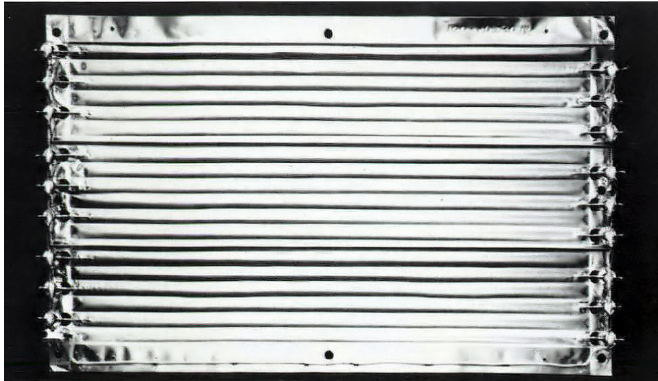
Figure 3. Panels of pressurized gas cells were mounted on the back of the main antenna for the purposes of detecting meteoroids; particles larger than 10^{-9} g could puncture Pioneer 10's cells and cause a detectable drop in gas pressure.
