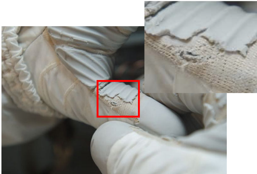
Figure 23. Damage on an EVA glove caused by pitting of an International Space Station handrail by meteoroids or orbital debris. This damage was photographed after EVA #3 of STS-118. Image taken from figure 4 of Christiansen and Lear (2013).
