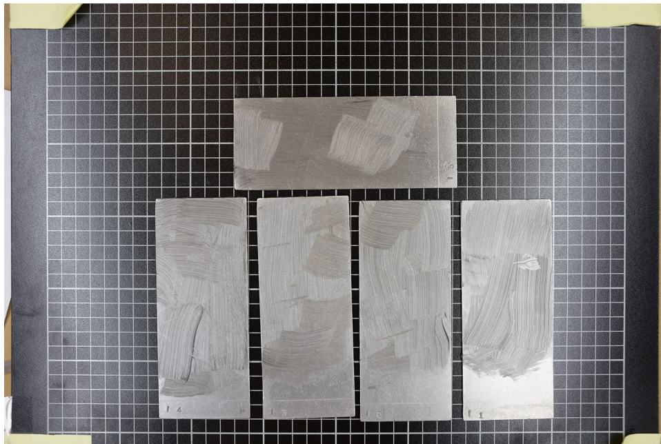
Figure 76. Method 4, Premalube, panels 1–5, before cleaning.
