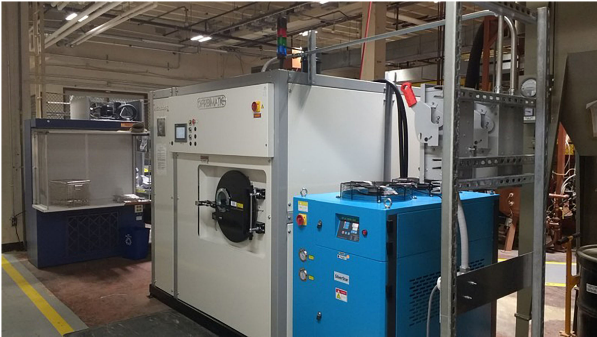
Figure 1. Firbimatic Multisolvent 50-volt vacuum degreaser.
