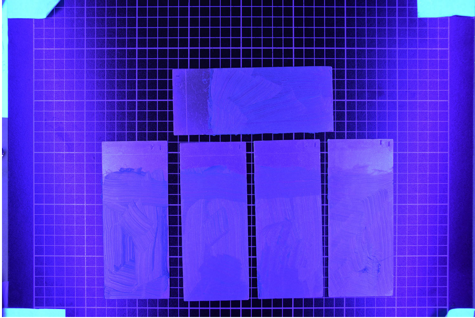
Figure 30. Method 2, Premalube, panels 1–5, before cleaning, UV light.
