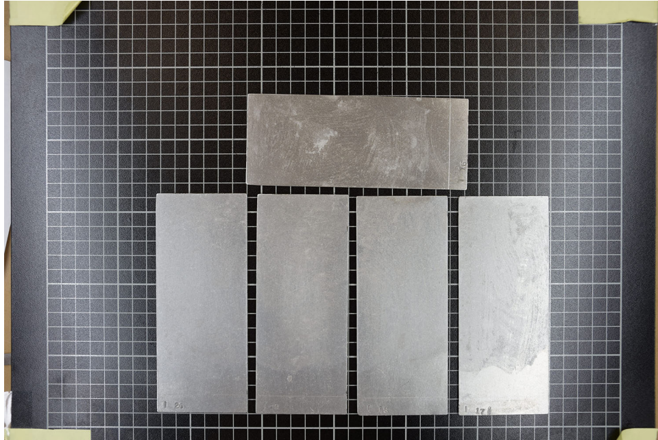
Figure 88. Method 4, synthetic sebum, panels 16–20, before cleaning.
