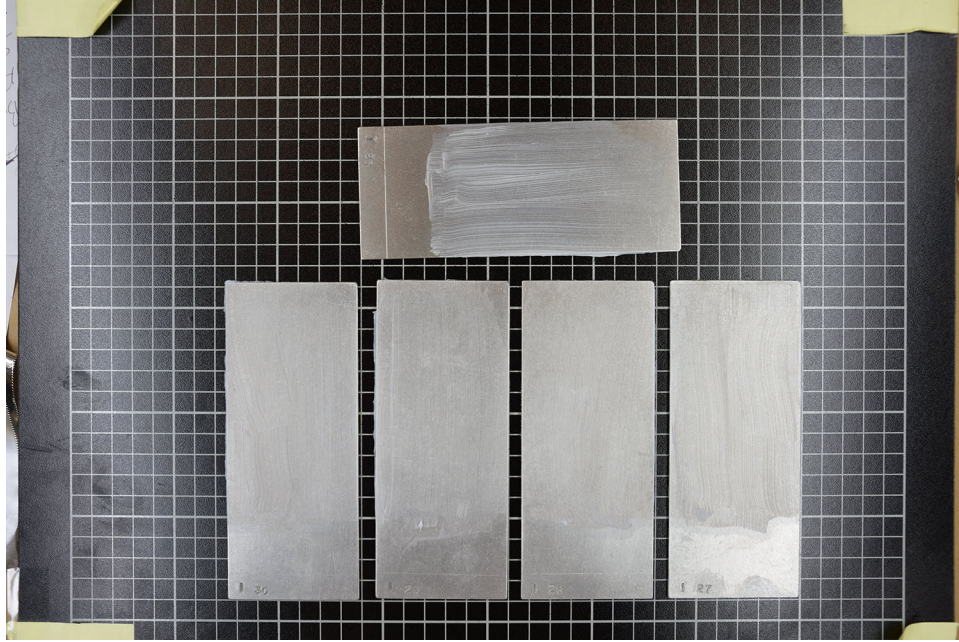
Figure 72. Method 3, Krytox, panels 26–30, before cleaning.
