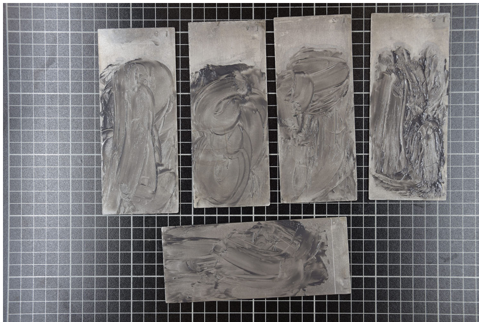
Figure 4. Method 1, Premalube, panels 1–5, before cleaning.
