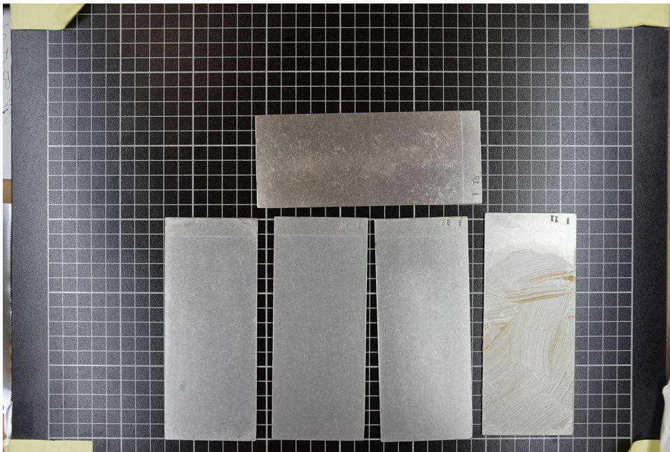
Figure 37. Method 2, AeroShell, panels 11–15, after cleaning.
