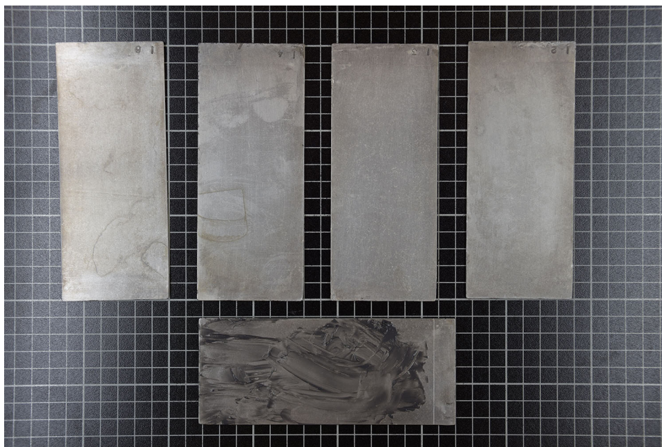
Figure 5. Method 1, Premalube, panels 1–5, after cleaning.
