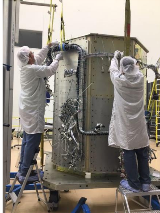
Landsat 9 Installing Harness
