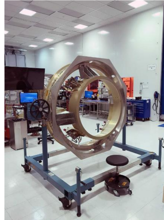
SC prop/rocket engine modules with thrusters on LVA. Inner ring is prop tank support ring. REMs/thrusters mounted around the outside of that. Outer ring is LVA.
