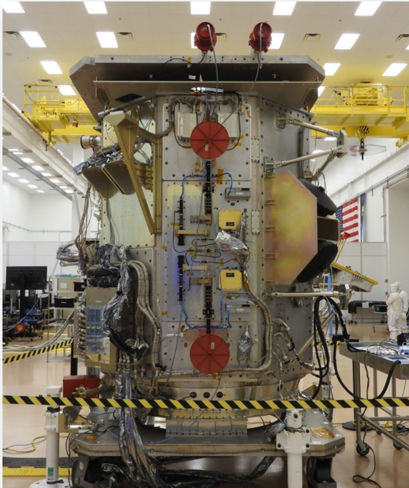
Landsat 9 spacecraft bus structure being assembled at Northrop Grumman Innovation Systems in Gilbert, AZ
