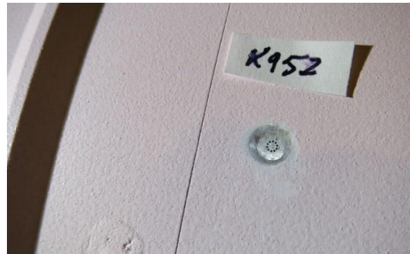
Figure 24: Transducer K952 After Sanding Treatment
