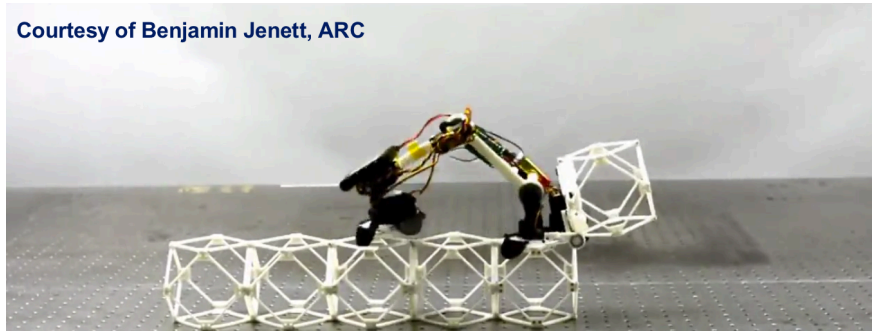
Figure 1. A robot (BiLL-E) assembling lattice structures
