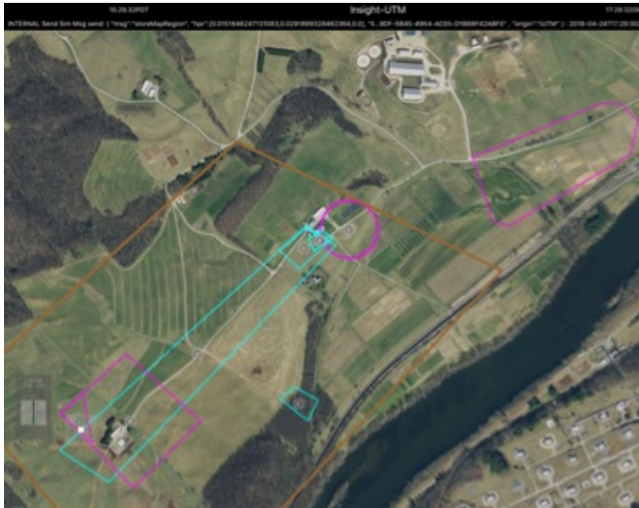
Figure 5. Example of a more complex scenario with 5 vehicles and more than one USS. Note: Magenta polygons are active volumes, cyan polygons are accepted volumes and the brown area is the USS client coverage area. The position of an airborne UAS is visible in the lower left corner/volume.
