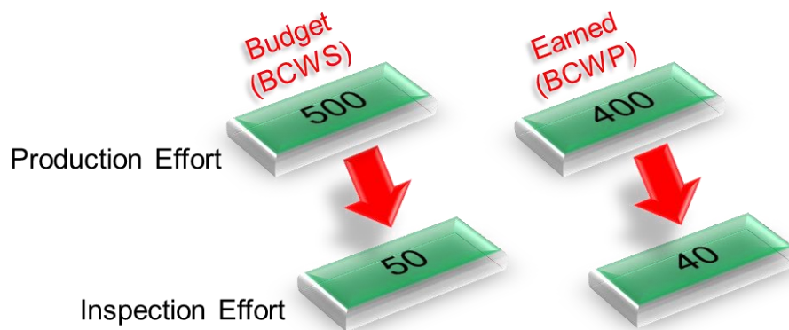
Figure 7. In the Apportioned PMT, the value for the AE (Inspection effort in this example) is based on (or apportioned to) the EV of the reference base task (Production effort in this example).
