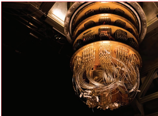
A dilution refrigerator for Google’s quantum computer. Image courtesy of Erik Lucero, Google
