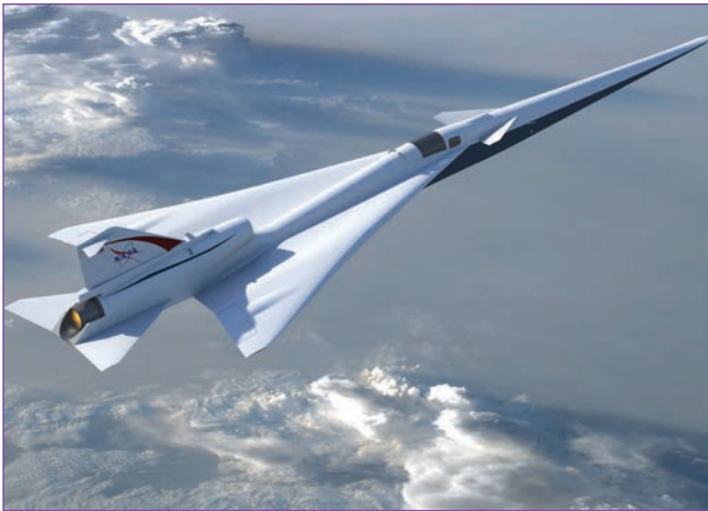
Illustration of NASA's planned Low-Boom Flight Demonstrator aircraft. The close proximity of the tail cone surfaces and jet motivated the work of jet surface interaction noise prediction (for example, jet scrubbing noise) with the use of hybrid Reynolds-averaged Navier Stokes/Large-Eddy Simulation methods. NASA, Lockheed Martin
