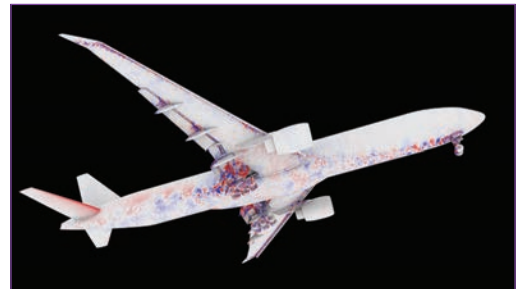
The fluctuating surface pressure resulting from the flow field around a large airliner produces broadband sound that propagates to the ground. Red denotes positive pressure fluctuations and blue denotes negative pressure fluctuations. Benedikt Koenig, Dassault Systemes; Patrick Moran, NASA/Ames
