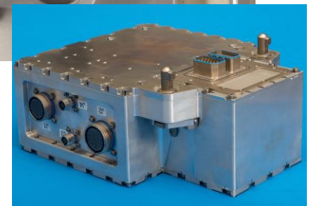
UEI Data Cube and Custom Sensor Supply Printed Circuit Board [Signal Conditioning and Power Distribution]
