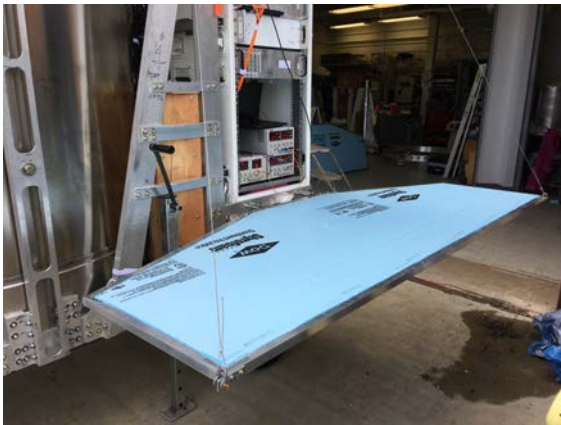
(a) Port Earth shield in deployed position
